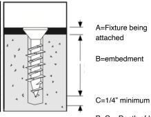
B+C = Depth of hole drilled
